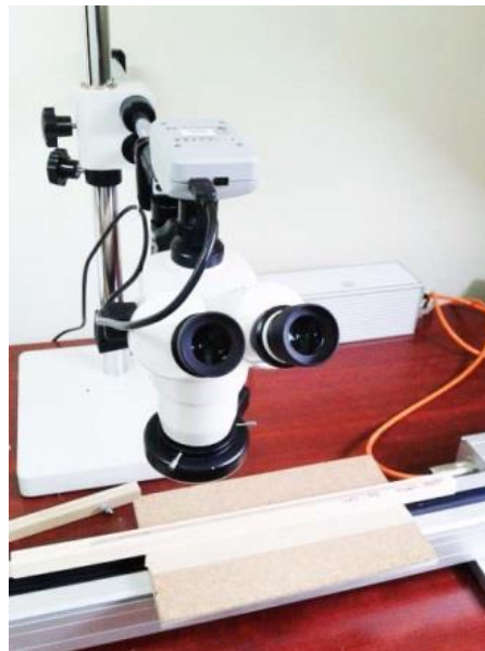
Figure 2 ATRICS system for scanning of wooden cores
