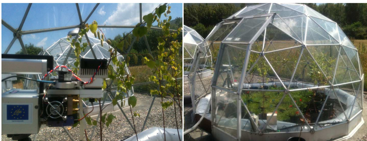
Fig.3. Sampling BVOC through LI-COR 6400 in the solardome
